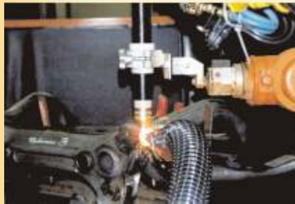
Final cut at a welded vehicle frame construction (IHU-profiles)
